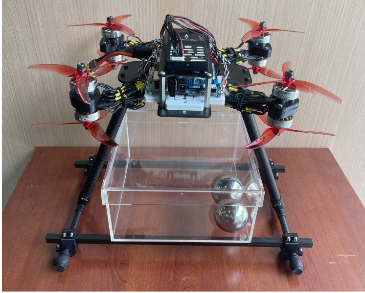
Fig. 6 X8-copter, whose detailed CAD model, shown in Figure 1, has been employed for high-fidelity simulations. As in the numerical simulations presented in this paper, two steel balls of 50.8 mm diameter are placed in a transparent rigid container that serves as payload compartment
